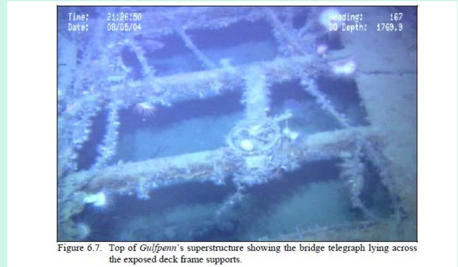
Figure 6.7. Top of *Gulfpenn*'s superstructure showing the bridge telegraph lying across the exposed deck frame supports.
